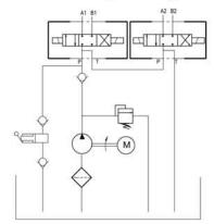
This power pack controls two independent functions on the hydraulic system but also has the manual override on both directional valves and integral hand pump in case of power failure.
